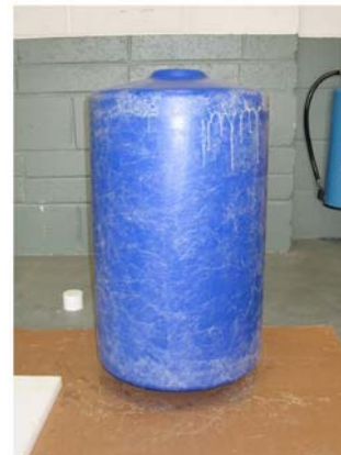
This shows the drum after spraying with adhesive.
