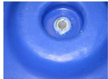
The new drum has a welded axle shaft.
